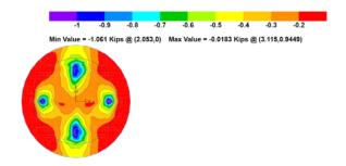
Figure 9: Finite Element Stress Results (4-Pile Cap)
