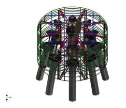
Figure 8: 3D Modeling of Concrete Cap Reinforcing (8-Pile Array)
