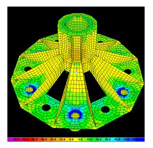
Figure 5: Stress Predictions From Finite Element Modeling
