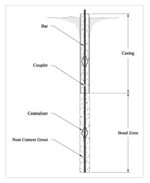
Figure 4: Composite Micropile Detail
