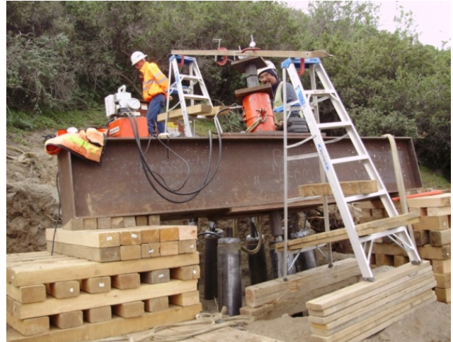
Figure 10: Typical proof test setup
