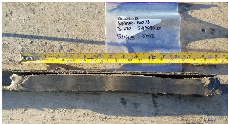
Figure 7: SPT sample at structure 670 from 27.5 m (90 ft) with soft glacio-lacustrine clay recovered in sampler.
